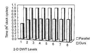
Fig. 16. Computing time of the proposed architecture and the parallel filter architecture for different 2-D DWT levels.
