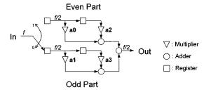
Fig. 10. Decimation filter employing the polyphase decomposition technique.
