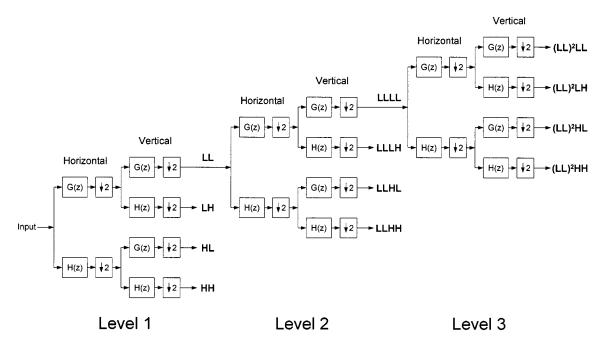
Fig. 1. Three-level 2-D DWT.
