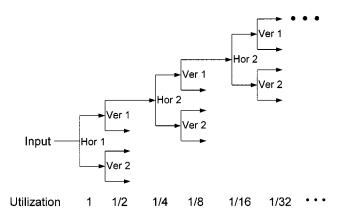
Fig. 6. Job allocation of the parallel filter architecture.
