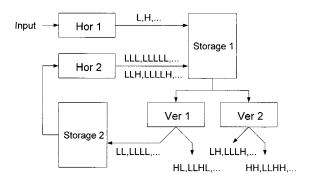
Fig. 5. Parallel filter architecture.
