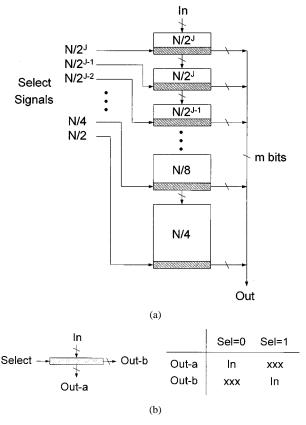
Fig. 13. (a) Line delay with select signals to change its size to N/2, N/4, N/8,...,  $N/2^J$  in the different decomposition levels. (b) The 1 to 2 demultiplexer used in the line delay.
