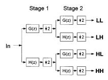
Fig. 8. Tree-structured transform module
