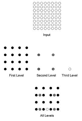
Fig. 4. MRPA for the 2-D DWT.
